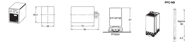
→<sup>1</sup>6<sup>|</sup>→ t=0.3 Note: PFC-N8 Mounting Bracket (provided with the Level Controller)
