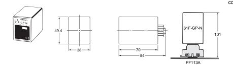
When mounting a Display Unit to a PF113A Surface-mounting Socket, secure the PF113A with the groove facing toward the bottom and then connect the 61F-GP-N the PFC-N8 accessory. **PFC-N8**
