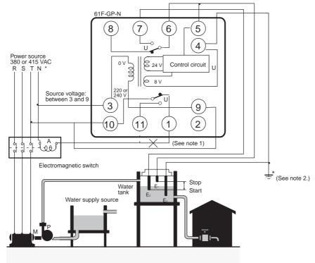
Note: 1. The diagram shows the connections for the water supply. When draining, change the connection from terminal 1 to terminal 11.2. Be sure to ground terminal 4.
